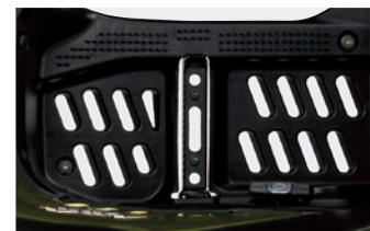
Full floorboards with drain holes
